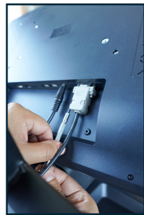
Connect the RS232 Plug into the correlating port, and tighten the screws on the plug with a very small flathead screwdriver.
