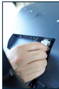
Connect the RS232 Plug into the correlating port, and tighten the screws on the plug with a very small flathead screwdriver.
